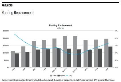
Remove existing roofing to bare wood sheathing and dispose of properly. Install 30 squares of 235-pound fiberglass asphalt shingles (min. 25-year warranty) with new felt underlayment, galvanized drip edge, and mill-finish aluminum flashing. Assume a 5-square hip roof; custom flashing at two average-sized skylights; and custom cap treatment at vented ridge.
